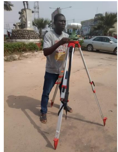
Fig. 6: Rover Receiver at One of the Selected Points (RR01) at Ring Road
