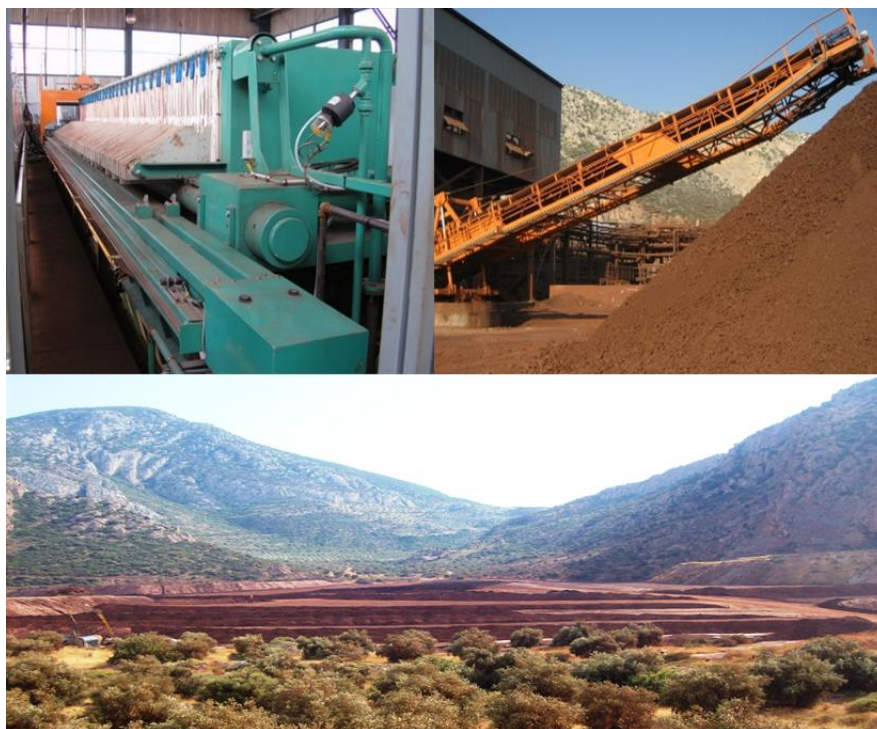
Figure 1. Filter press in operation and BR discharge (above); site of BR disposal in the plant (below)
