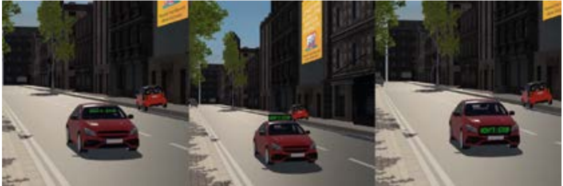
Caption: Various ways to display the intent of an oncoming vehicle through the use of visual signs
