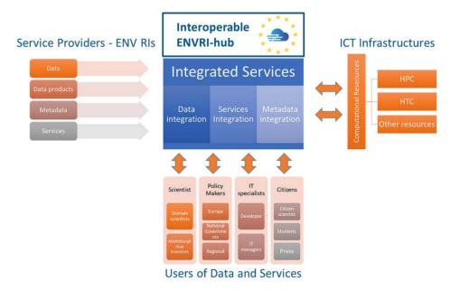
Figure 2.4: The ENVRI-hub Architecture [17]
