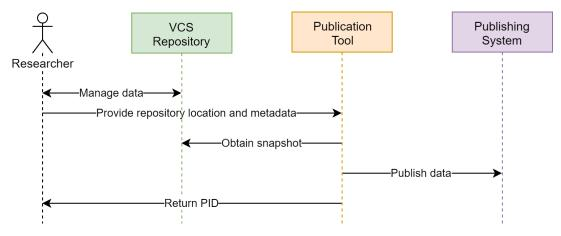
Figure 3.1: Data publication workflow using the proposed tool
