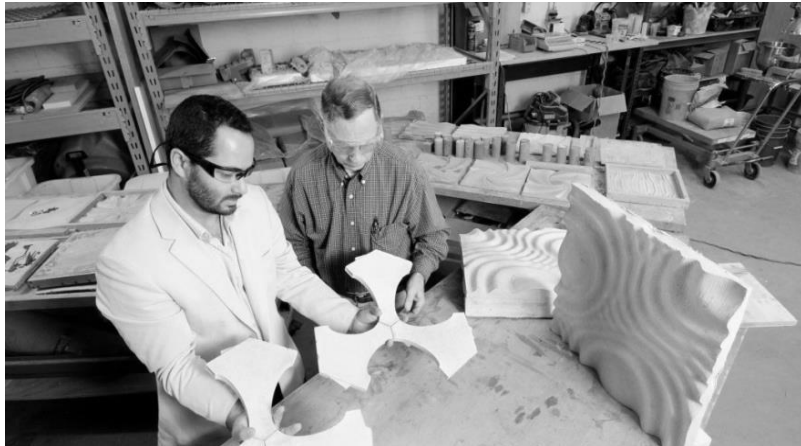
Fig.2:- Computer to Construction: Technique Enables Mass Production of Custom Concrete Building Components from Digital Designs. (Source: https://precast.org/2013/04/liquid-walls/ , date accessed: 03 Dec, 2019)
