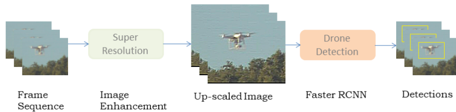
Figure 2. Drone detection pipeline with SR
