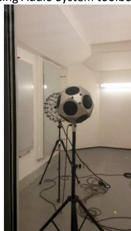
Fig 3.3. Measurement SPL and reverberation time with acoustic camera in large number of positions
