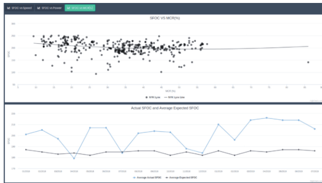
Figure 6: Inefficiencies using SFOC scatter
