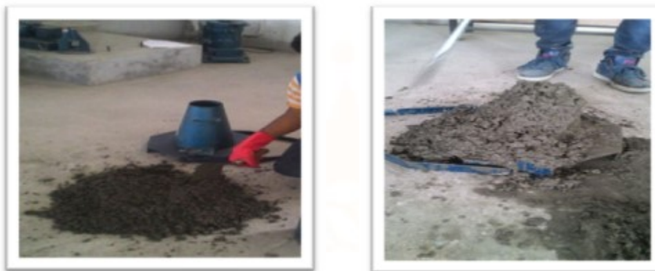
Figure 6: slump value test
