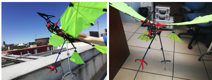
Fig. 7. Two claws on an ornithopter used for the project GRIFFIN an european ERC advanced grant
