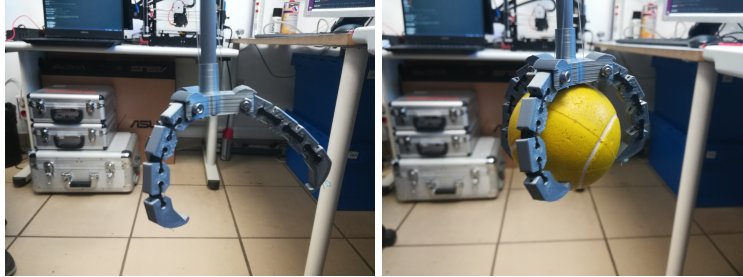
Fig. 6. Grasp of a plastic ball by the three finger of the claw, it can be observed that the claw can put up with the weight even looking downwards
