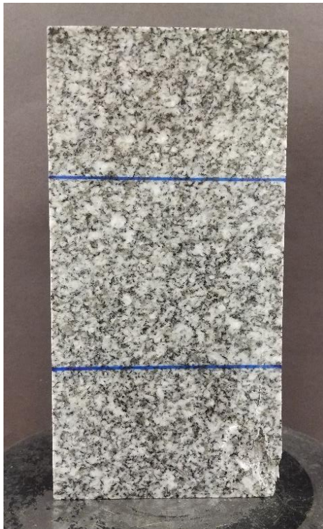
Figure 6. Barre Granite Specimen at failure
