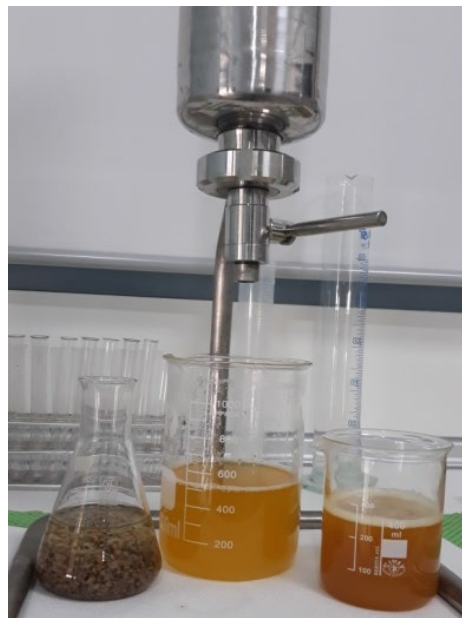
Fig.1. Opuntia ficus indica extracts after maceration and percolation process; from left to right: extracts from unripe fruit seeds (in conical flask), from leaves and fruit peels (large beaker with light colored liquid), and from ripe fruits containing their seeds (smaller size beaker), respectively.
