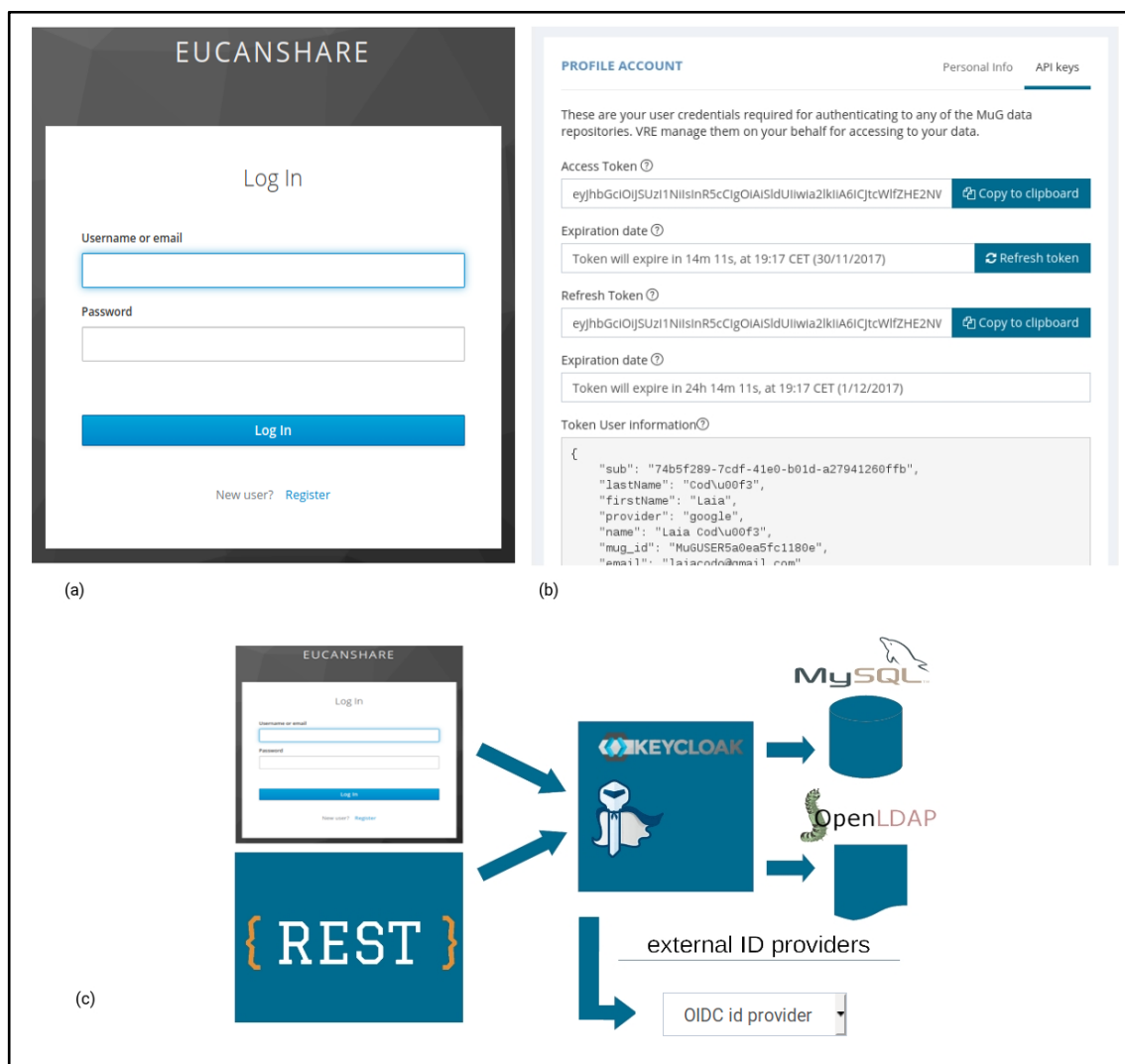
Figure 7. (a) EuCanSHare Login page. (b) User profile details including authorization tokens. (c) Schema of the centralized authorization service based on Keycloak.
