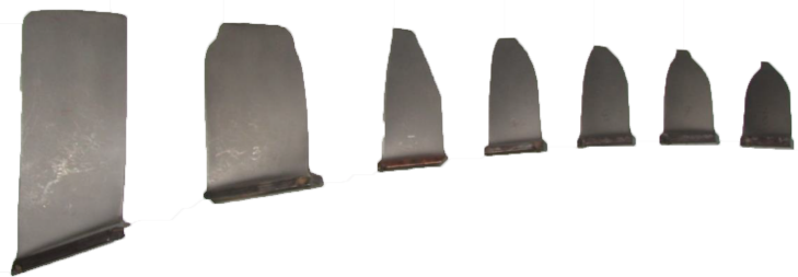
Figure 2. Erosive wear of compressor blades.
