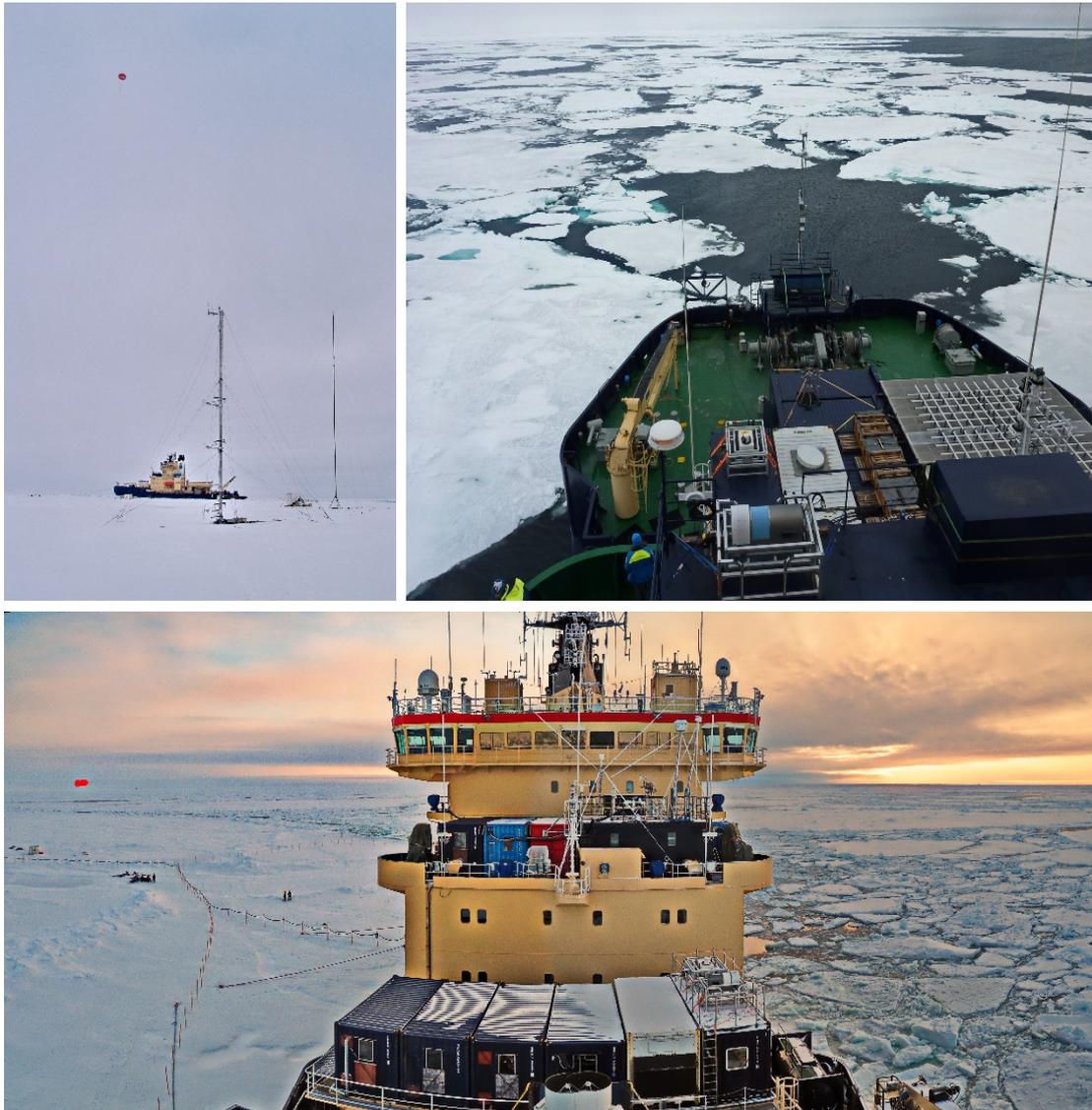
**Figure 1.** *Top left: Oden during ASCOS with micro-meteorology masts and ocean site in foreground. Top right: Foredeck of Oden during ACSE, with cloud and wind radars, scanning lidar and microwave radiometer and the bow mast for eddy covariance fluxes in the background. Bottom: Oden viewed from the top of the bow mast during AO2018, with similar instruments on the foredeck (scanning cloud radar and lidar, and radiometer) and a suite of atmospheric observations on the top 7<sup>th</sup> deck.*
