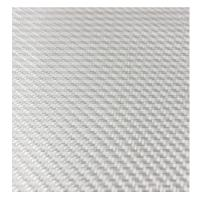
Fig. 1 Bidirectional fiberglass
