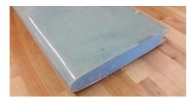
Fig. 4 Complete wing core with fiberglass skin
