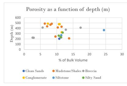
Fig. 1 Porosity of the Ross River well core samples as a function of depth, separated by lithology
