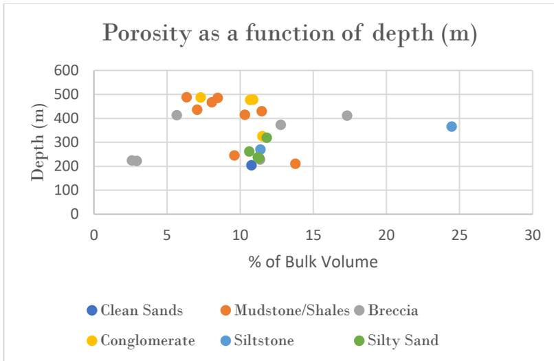
**Fig. 1** Porosity of the Ross River well core samples as a function of depth, separated by lithology
