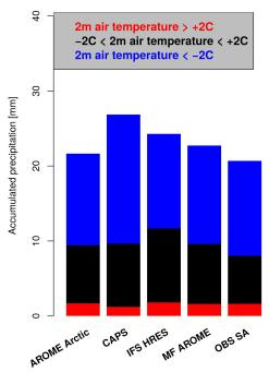
Accumulated precipitation (estimated by temperature thresholds; rain in red, sleet in black and solid precipitation in blue) for AROME Arctic, CAPS, IFS HRES, AROME MF with lead times +18 to +42hr, observed precipitation from Geonor rain gauges with single alter shields
