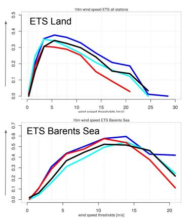
Equitable Threat Score (ETS) and Frequency Bias (FB) for wind speed over all synop stations used in the model-intercomparison. Models are IFS HRES (red), AROME Arctic (blue), CAPS (black) and AROME MF (cyan). Lead times from +25 to +48hr.
