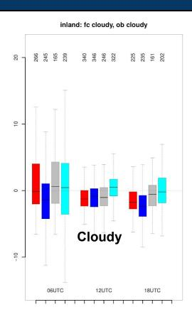
Conditional verification of T2 for inland stations. Box-and-whiskers plot of T2 errors (forecasted minus observed) conditioned by TCC (4 boxes to the left) and conditioned by wind (4 boxes to the right). Each box is divided into models and time of day. Number of cases is plotted at top and outliers is omitted to increase readability in plots.
