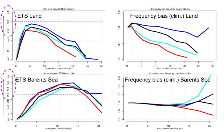
Equitable Threat Score (ETS) and Frequency Bias (FB) for wind speed over all synop stations used in the model-intercomparison. Models are IFS HRES (red), AROME Arctic (blue), CAPS (black) and AROME MF (cyan). Lead times from +25 to +48hr.
