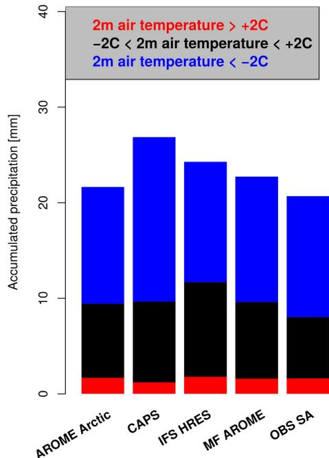
Accumulated precipitation (estimated by temperature thresholds; rain in red, sleet in black and solid precipitation in blue) for AROME Arctic, CAPS, IFS HRES, AROME MF with lead times +18 to +42hr, observed precipitation from Geonor rain gauges with single alter shields
