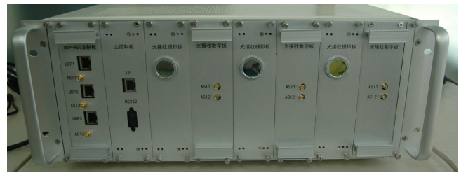
Fig. 9. The actual object of the optical receiver.
