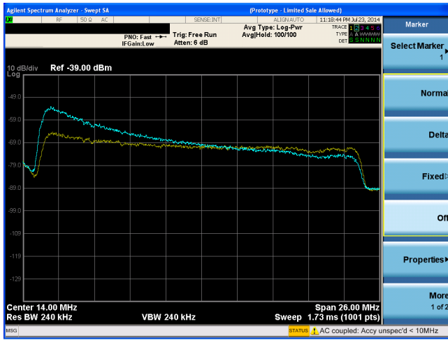
Fig. 5. Spectrum of the received signal without pre-distortion: blue curve. Spectrum of the received signal with pre-distortion: yellow curve.
