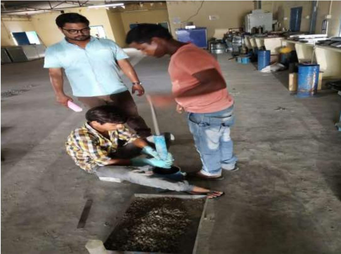
*Fig.1:- CBR Test of Ferrochrome slag mixed with red soil*
