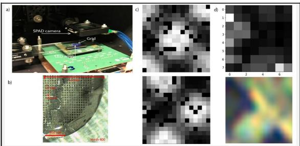
Fig. 1: (a) Microscope setup. (b) Grid used for observation. (c) Shadows obtained on the SPAD camera for (top) LED (0,0) and (bottom) LED (4,0). (d) LED Image: composition obtained taking one SPAD signal and linking it to each LED. On the bottom is the grid oriented and sized similar.
