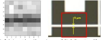
Fig. 2. An image taken with our microscope (left) of a line pattern of 5  $\mu m$  width. In the right it is shown an image taken with a conventional microscope.
