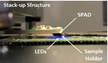
Figure 1. Microscope setup showing LEDs, the Sample Holder with an EBL sample in it and the SPAD detector.
