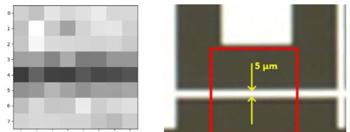
Fig. 2. An image taken with our microscope (left) of a line pattern of 5  $\mu\text{m}$  width. In the right it is shown an image taken with a conventional microscope.
