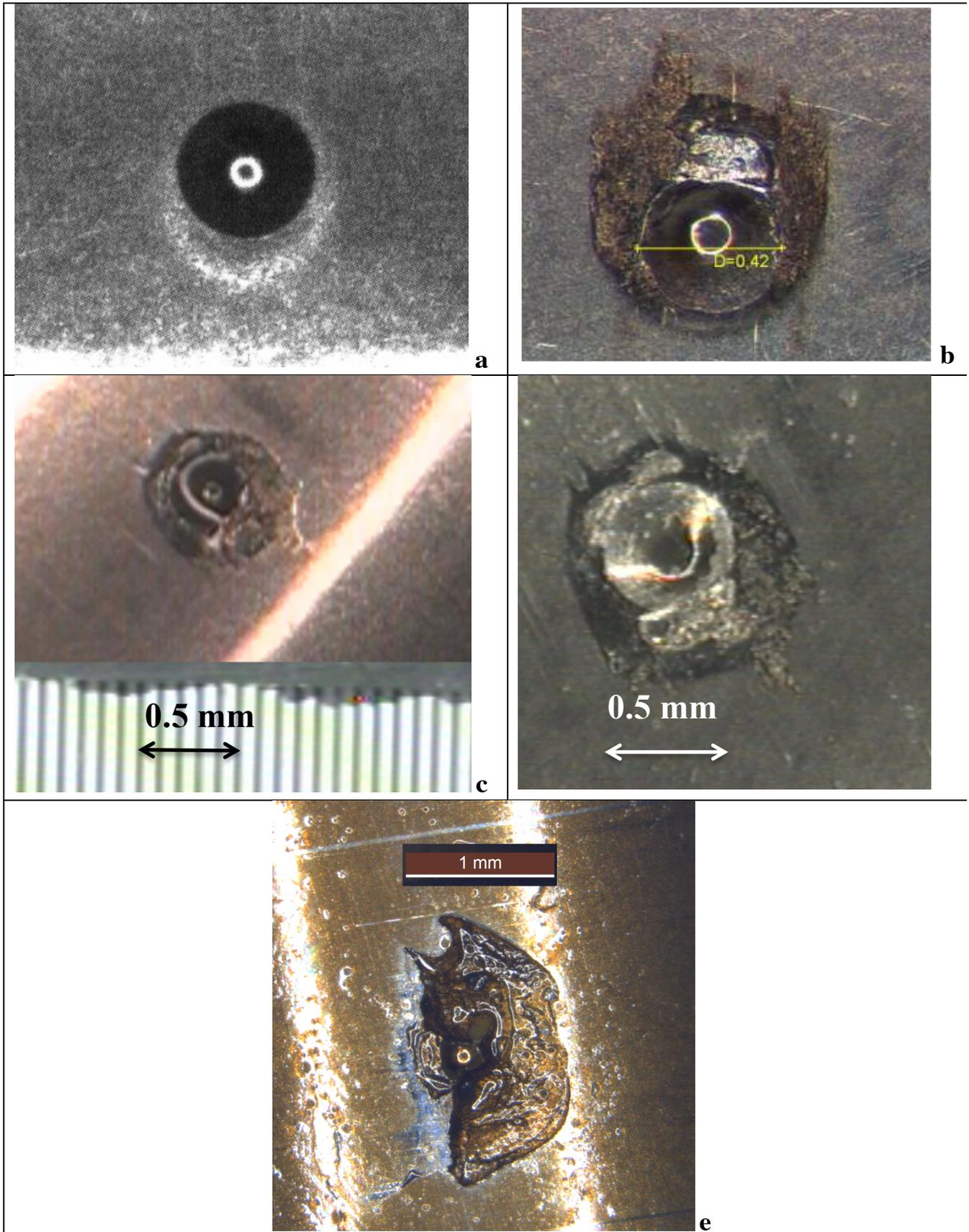
Figure 3: the progression of the indentation of bearing 4A; a) initial defect; b) after 19 hours at various load and speed conditions; c) after 70 hours ; d) after 124 hours; e) after 332 hours – c), d) and e) at 300 rpm and 1800 N
