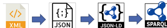
Figure 10. Conversion flow of data format from XML to JSON to JSON-LD to enabling SPARQL queries
