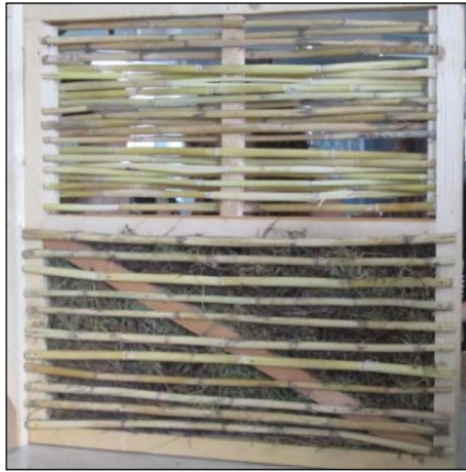
Figure 2.5: Wattle & Daub wall constructed in the laboratory of NTUA.
