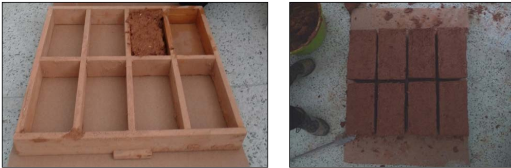
Figure 2.4: Experimental adobe bricks produced in the laboratory
