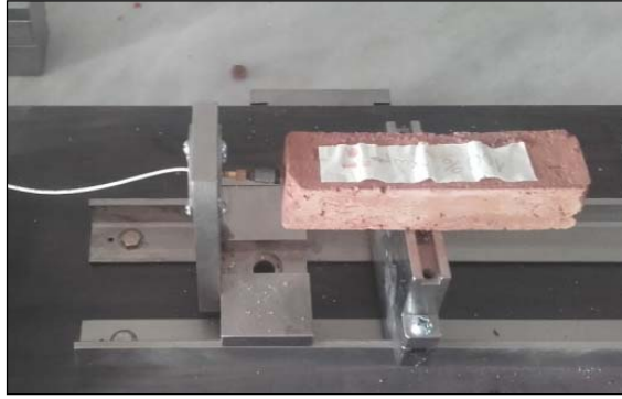
Figure 5.12: Experimental arrangement of the dynamic modulus E
