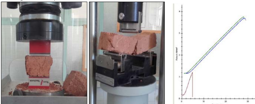
Figure 5.11: Experimental devices and results of compressive strength and bending of three points of Earth mortar
