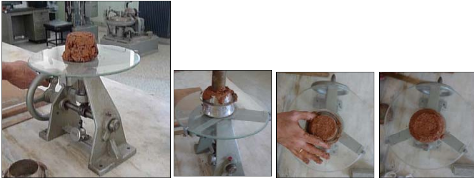
Figure 5.8: Testing the specimen in the spreading bank
