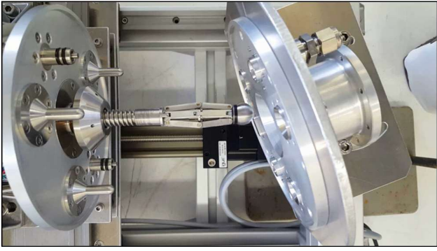
Fig. 1. ASSIST breadboard, photo ESA courtesy. The docking fixture is shown in the right part, and the docking end effector in the left part.
