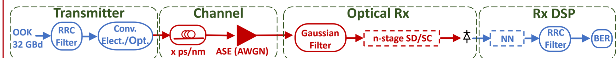
Fig.3 - Simulation setup. Reference system without the dashed blocks. RRC: root-raised cosine.
