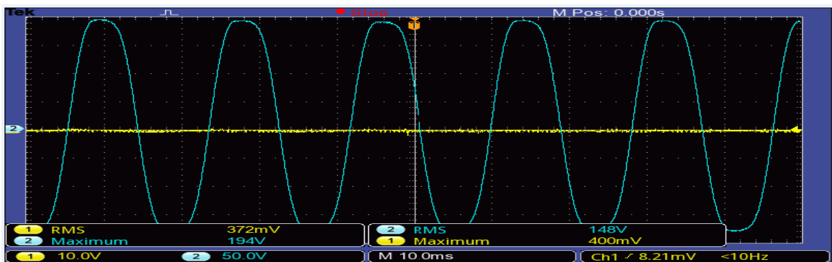
Figure 13: The steady state of filtered voltage output of the proposed system.
