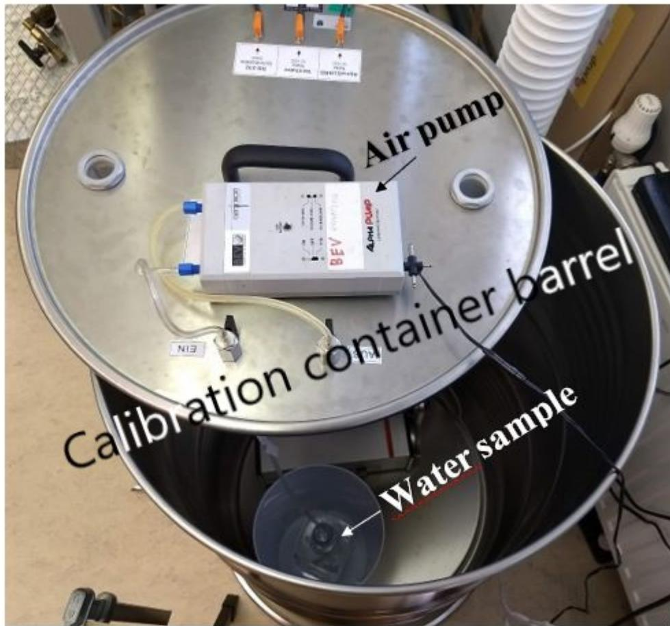
**Figure 1.** Radon calibration container with a drinking water sample together with the Austrian national standard ionisation chamber for radon 222 activity concentration in air inside and the air circulation pump outside the calibration container barrel
