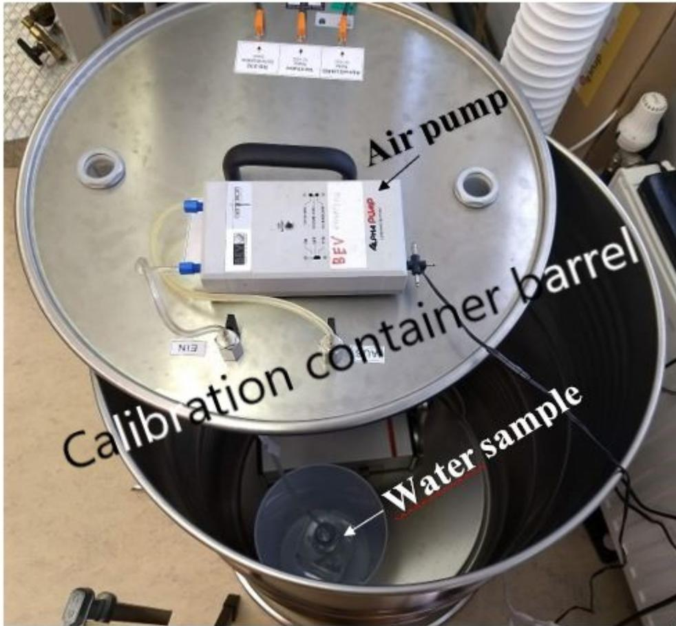
**Figure 1. Radon calibration container with a drinking water sample together with the Austrian national standard ionisation chamber for radon 222 activity concentration in air inside and the air circulation pump outside the calibration container barrel**
