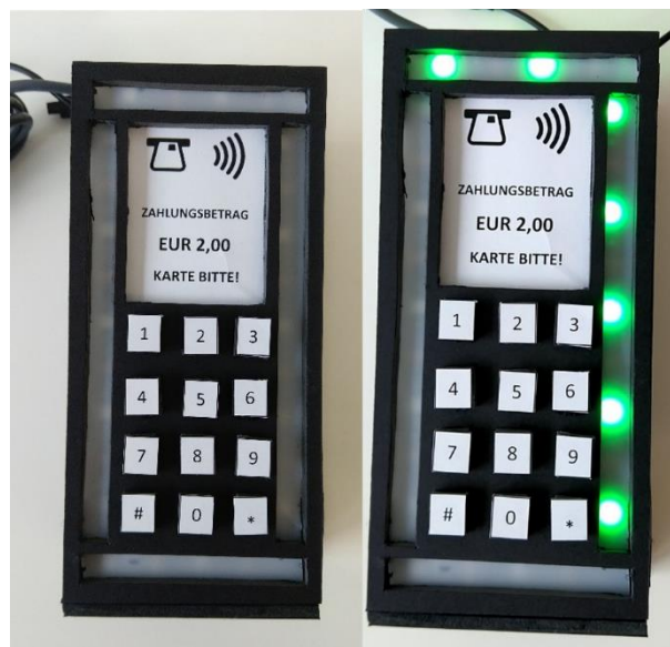
Fig. 2. a) Visual feedback prototype b) visual feedback prototype with LEDs lighting in a clockwise direction to indicate the state of the transaction
