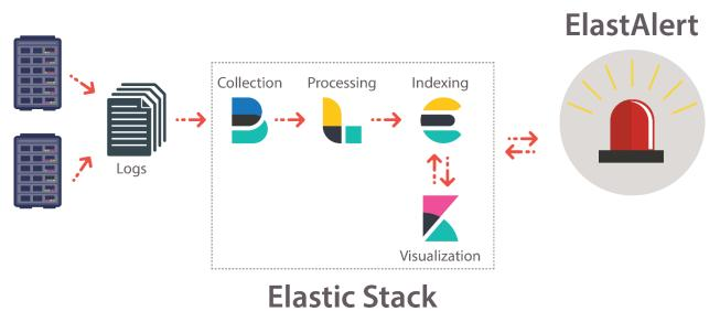
Figure 1. Log management in IT-DB and monitoring with ElastAlert
