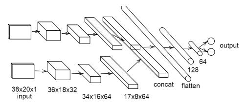
Fig. 5: 2D classification network with 2 inputs.
