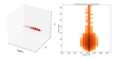
Fig 1.(From left to right) a) 3D visualization of energy depositions. The size of the spheres is proportional to the energy in the cell. b) Total energy of all trigger cells
