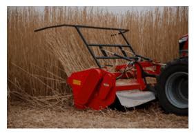
Figure 6.2 – shredder attached to the front PTO of the tractor
