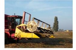
Figure 10.4 - Modified combine with elevation system for wheat header
