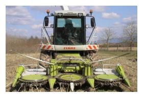
Figure 1.3 – Class Jaguar SPFH with kemper type header
