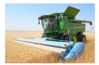
Figure 2.3 – header with stripping rotor
