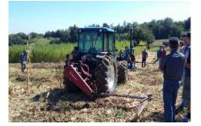
Figure 10.5 - Cutting bar to be used after threshing
