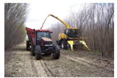
Figure 18.3 – self propelled forage harvester equipped with SRC header
