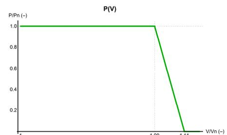
Figure 2. Autonomous P (V) function of smart PV inverter
