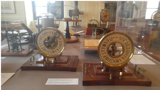
Fig. 1. The alphabetic telegraph transmitter and receiver exhibits in the Scientific Instruments Gallery of the History Museum of the University of Athens.
