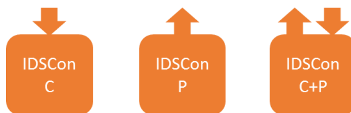
Figure 5. Three types of IDS Connectors defined for Z-BRE4K: for Data Consumer (left), Data Provider (middle) and Data Provider + Consumer (right)
