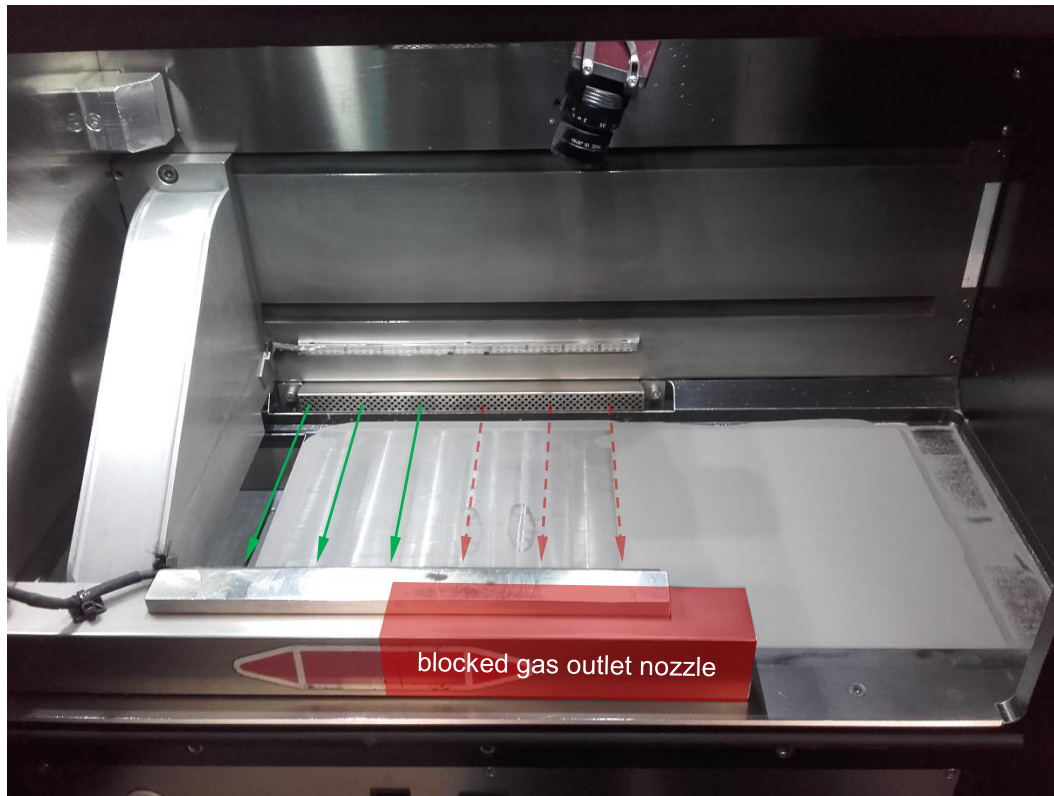
Figure 14: Inert gas flow direction and area of blocked gas outlet nozzle
