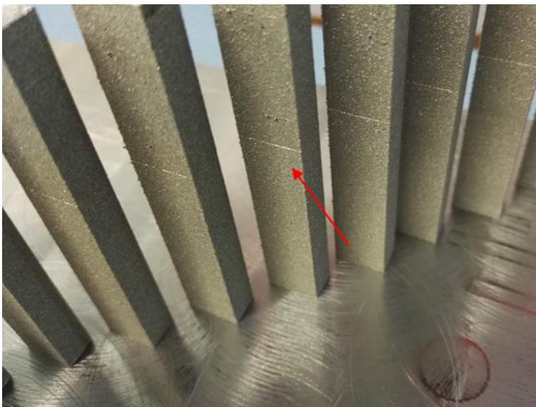
Figure 10: Marks caused by pausing a building job
