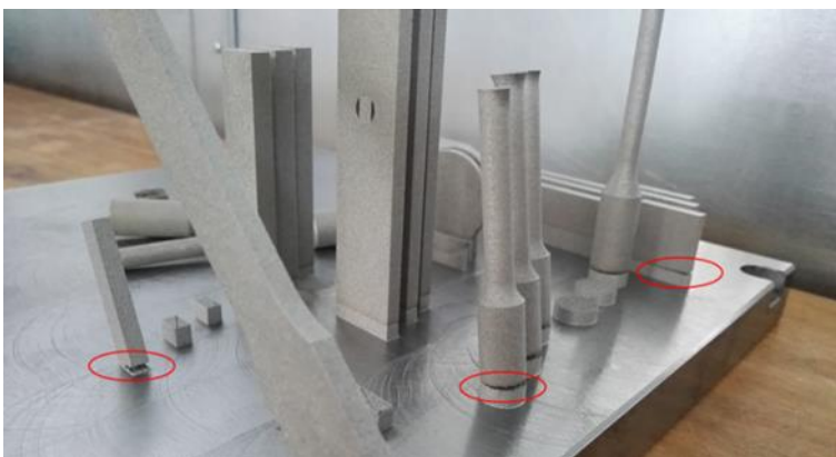
Figure 8: Break in the interface between support and component due to weak support strategy
