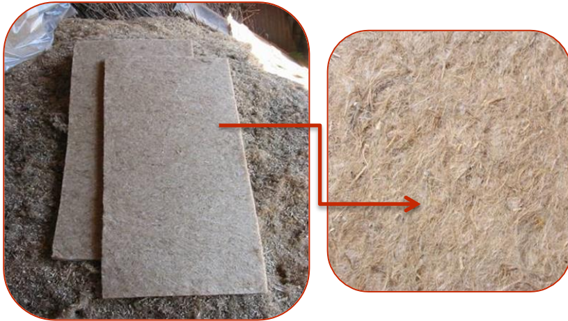
Figure 6: Insulation mats produced by KEFITALIA (BIOKENAF project)
