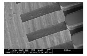
Figure 1: SEM image of PLLA cantilevers after chip release. The support structure is visible to the right.
