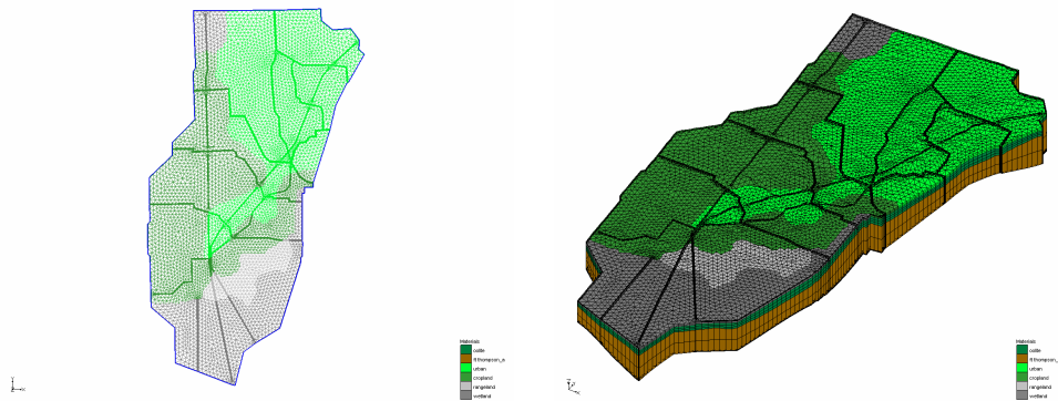
FIGURE 2. The computational mesh of the coupled 2-D/3-D model: 2-D (left), 3-D (right).
