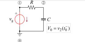
Figure 1: Simple capacitor circuit.
