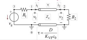
Figure 5: Transmission line circuit; the Laplace transform domain.
