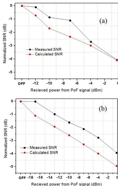
Fig. 4 Normalized calculated SNR and  $\text{SNR}_{\text{decode}}$  vs. PoF power delivered at reception stage with data signal power of: (a)  $-8$  dBm (b)  $-12$  dBm.
