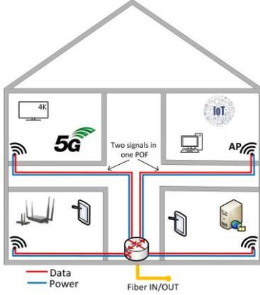
Fig. 1 Illustrative POF network for multi-standards wired and wireless transmission in the home applications with remote power delivery.
