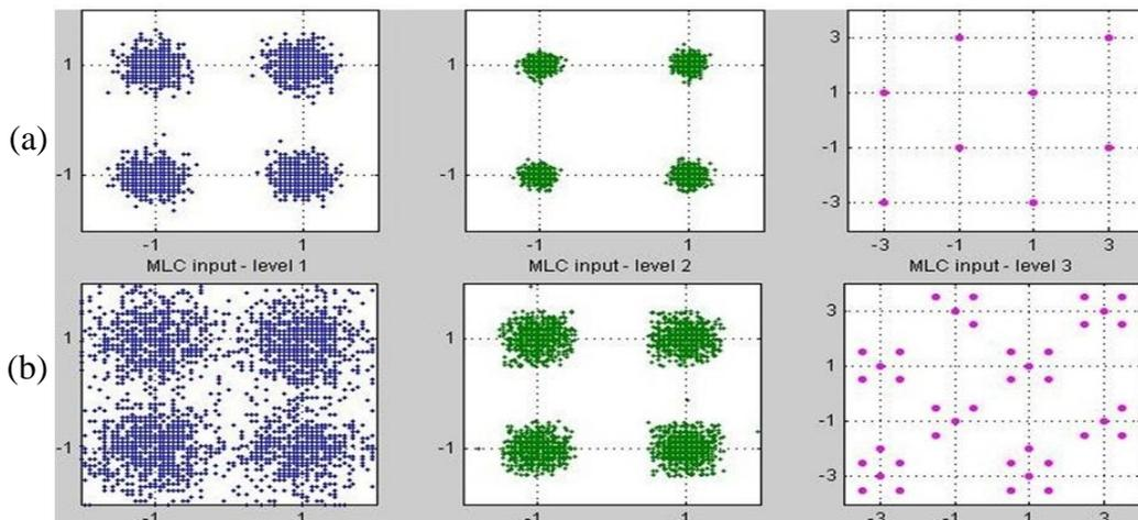
Fig. 5 Constellation diagram of the multilevel decoding inputs: (a) Only data signal, -8 dBm at PD. (b) Both data and power channels at PD; data -12 dBm, power -0.2 dBm.
