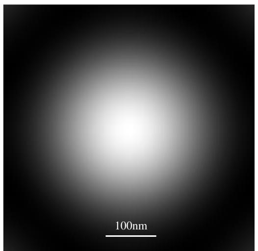
Thereby, points' images overlap and can not be resolved when they are close to one another. Existing Single-Point-Localization (SPL) techniques turn on adjacent molecules at different times.
