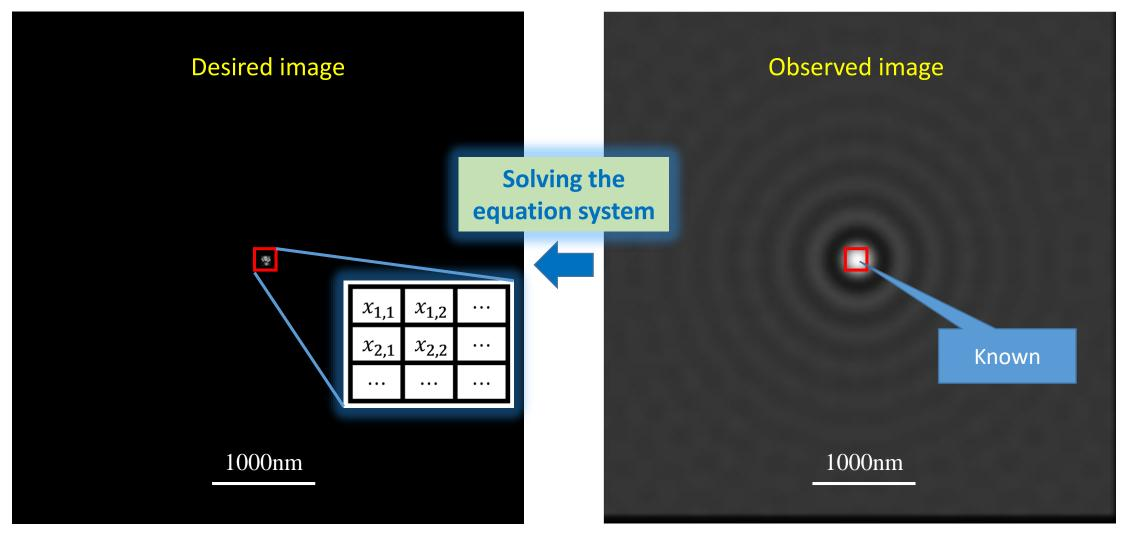
As a result, the desired image's ROI pixels are recovered by solving the equation system.
