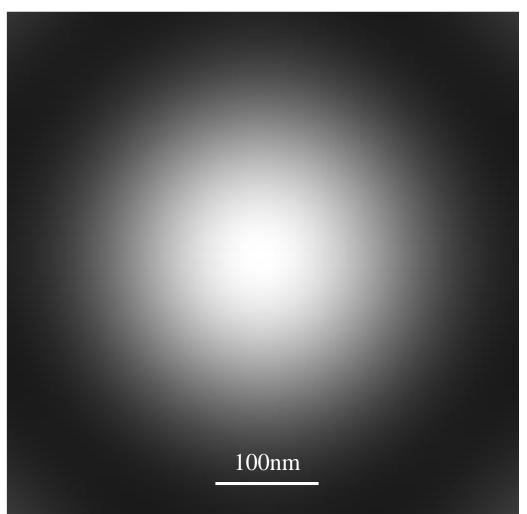
Imaging procedure can be modeled as the convolution of the structure with the PSF. These results are very blurred, look like the PSF. No structure can be observed directly.
