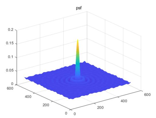
The PSF is known, and sometimes could be treated as a Gaussian Function. Thereby, the location can be figured out by data fitting, etc. (Unit of the coordinates: pixel)
