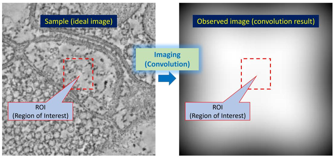
The ROI's light intensities are **submerged by extra lights** (the images of outside structures). This prevent the ROI from being figured out because the **extra lights are unknown**.
