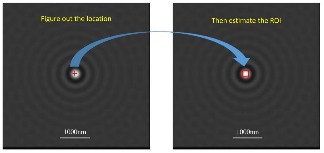
The ROI's size can be determined using prior knowledge, e.g., the molecule's maximum size.
