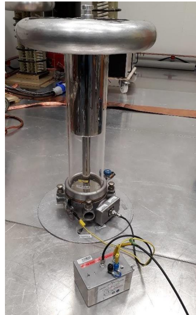
Figure 3: The 100 \text{ kV} capacitive voltage divider with active low voltage arm. High-voltage arm capacitance is 37 \text{ pF} and low-voltage arm 290 \text{ nF} .
