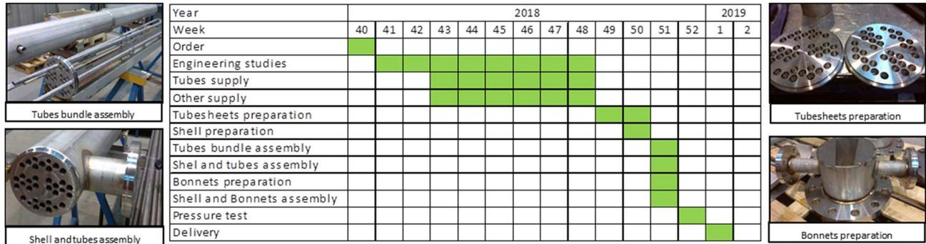
Figure 7: Illustrated planning of the test heat exchanger manufacturing
