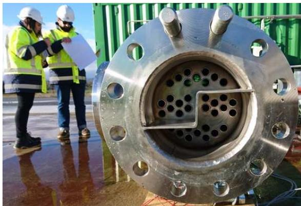
Figure 8: View of the test heat exchanger inspection before piping works.
