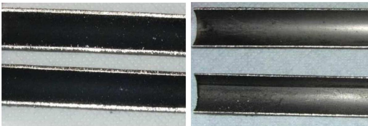
**Figure 3: Visual inspection of scales in 1.4571 (316Ti, left) and Ti Gr.2 (right) after 83 days of exposure in the hot temperature skid at Soultz-sous-Forêts.**
