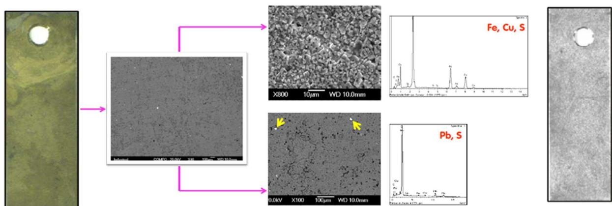
**Figure 5: View of one TI 35 coupon (right) and one Ti Gr.7 coupon (left) after 101 days of exposure and the results of Scanning Electronic Microscope analysis performed on scales.**
