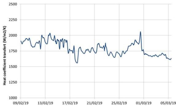
**Figure 10: Evolution of the heat transfer coefficient during the first week of test.**
