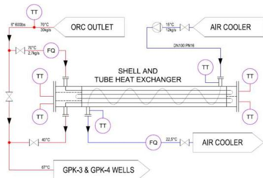
Figure 9: Simplified Piping and Instrumentation Diagram of the test heat exchanger pipes (TT, temperature sensor, FQ, flowmeter).
