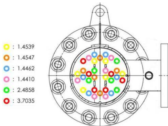
**Figure 4: Drawing of a tubesheets with the different tubes metallurgy selected.**
