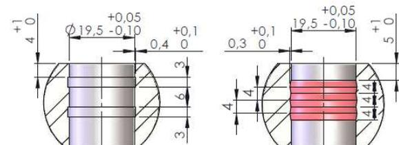
**Figure 6: Draft of the 2 square grooves for stainless steel and nickel alloy tubes (left) and the 3 triangular grooves for titanium tubes (right)**
