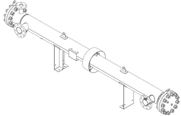
**Figure 3: Draft of the NEN design adopted for prototype heat exchanger**
