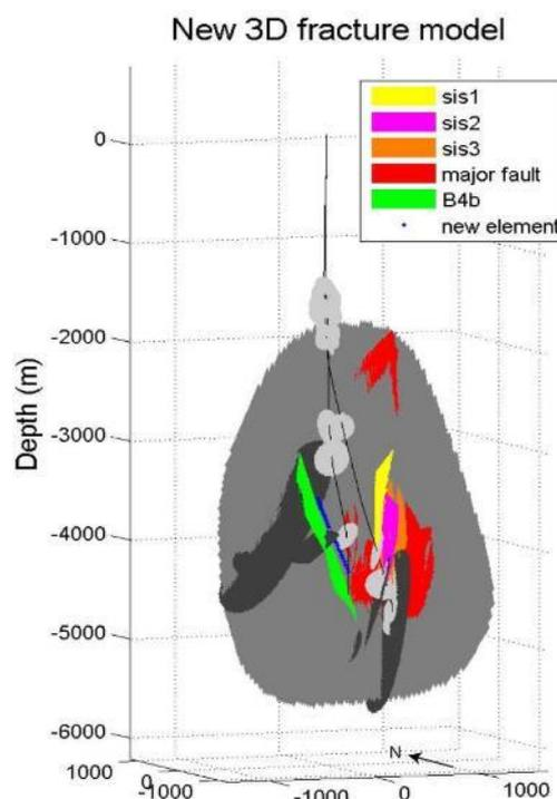
**Figure 8: 3D model of the main fracture zone/fault in the Soultz granite derived from VSP and geophysical data (micro seismicity, image logs) (Sausse et al., 2010, Lubrano, 2013)**
