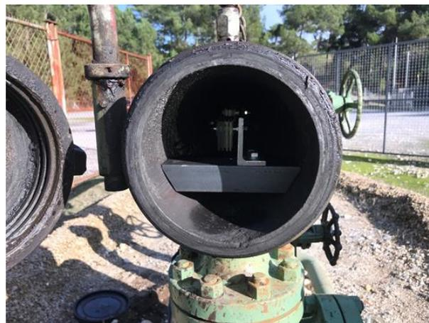
**Figure 4: a set of 7 coupons installed in a dedicated rack for corrosion study installed in a Cazaux oil well (Source: Vermilion)**
