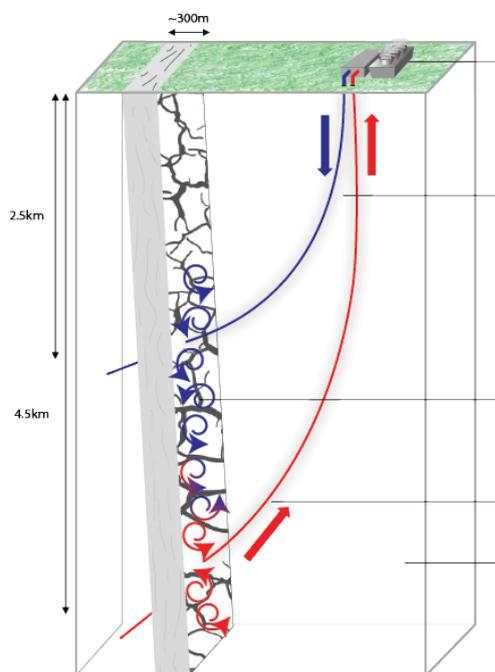
**Figure 7: Sketch of the geothermal doublet under drilling operation in a faulted granite at UDDGP site in Cornwall, UK (Law, 2018).**
