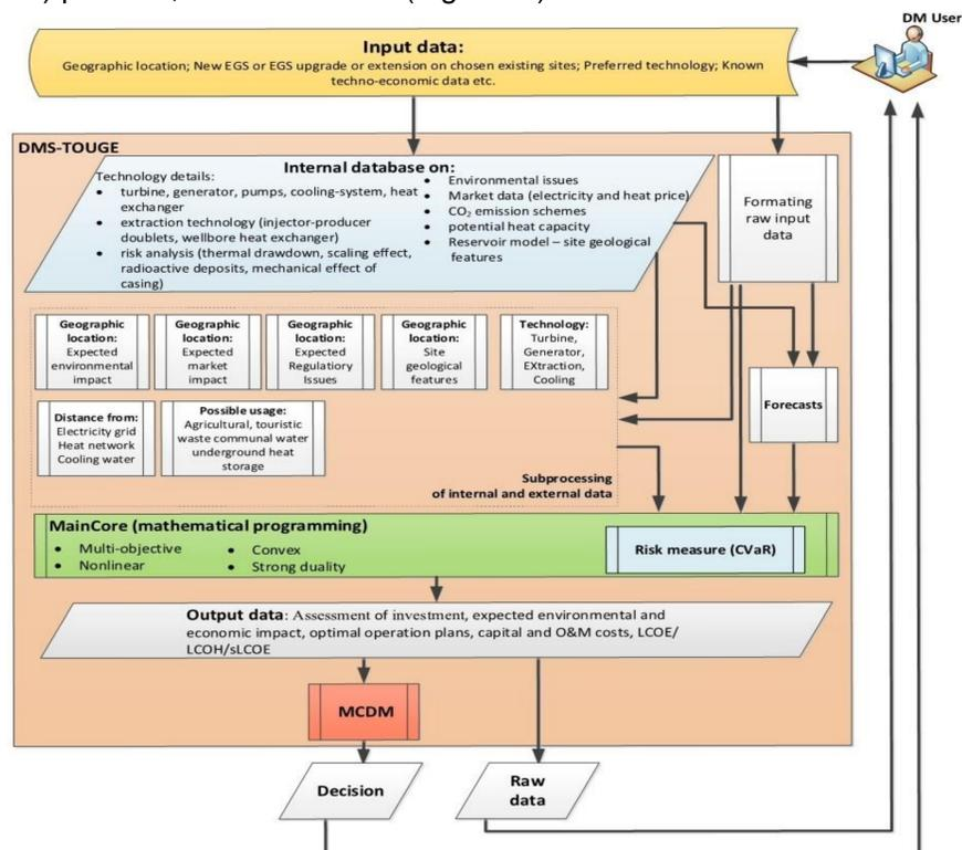
Figure 2. Schematic description of main processes in DMS-TOUGE
